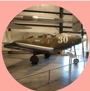
**The P-39 Airacobra** has several unique design features, including an engine behind the pilot, automobile-type doors, and tricycle landing gear. The P-39 had great performance at low altitudes, but was ill-suited to flying at high altitudes. The large 37 mm cannon mounted on the nose made them excellent ground attack aircraft however, and the US sent large numbers of P-39s to the Soviet Union under the Lend-Lease Act for this purpose.
