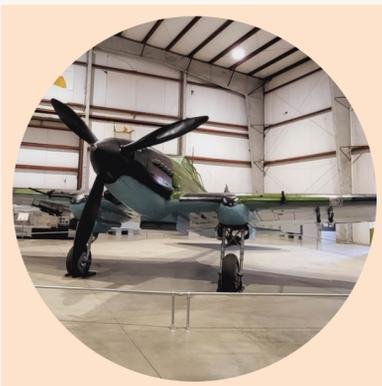
**The IL-2 Shturmovik** was a Soviet plane used for ground attack. Faced with a severe shortage of aluminum, the plane was built with its wings and tail section made from wood. The nose and cockpit were heavily armored, making them difficult to shoot down from the ground. They were vulnerable from the air however, and thousands were lost during the war. While not technologically advanced, the IL-2 became the most produced aircraft of WWII, with an estimated 36,000 of them built.
