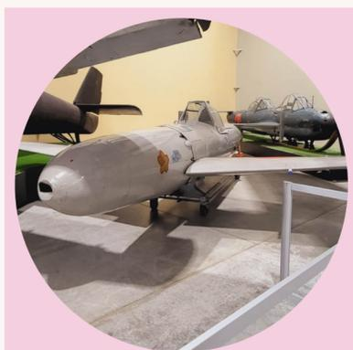
**The Ohka** is a Japanese human-guided bomb that was designed in 1944 for the purpose of attacking Allied warships. They were carried to within range of their targets beneath a Japanese G4M Bomber (codenamed "Betty"). Once released, the pilot would guide to bomb to the target. Being a suicide mission, the pilot would remain with the bomb upon detonation. Ohka's hit 7 U.S. ships, 3 of which sank. The success of the Ohkas were limited by the vulnerability of the Bettys that carried them.
