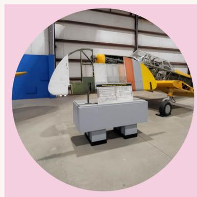
The display of the **Fabric Covering Process** shows how the museum would restore a fabric plane. Most early planes were made from fabric and wood. Even into WWII, some planes still included fabric elements in their design. One example is the British Hawker Hurricane (next page). The rear fuselage was made from fabric as were the wings in early versions of the Hurricane. Today, some gliders, homebuilds, and light sport aircraft are still designed with advanced fabric coverings.
