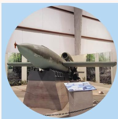
**The German V-1 "Buzz Bomb"** is the world's first operational cruise missile, meaning it was self-guiding and not radio controlled. They used a magnetic compass in their pre-set guiding system. The Buzz Bomb was first used operationally in June 1944 when the first V-1s were fired at London from France across the English Channel. The German's fired V-1s into Great Britain, killing an estimated 8,000 people, and mainland Europe, killing an estimated 4,600 people.
