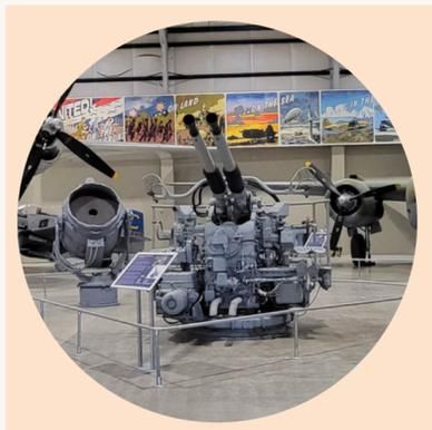
**The Twin Bofors 40mm** was one of the most widely used anti-aircraft weapons of WWII. Originally designed in Sweden, the US Navy acquired a license to build them with modifications including, converting the targeting units from metric to imperial, updating ammunition, powered mounts, and adding a liquid cooling system. By the end of WWII, Bofors 40 mms were found on almost every American ship. Some were used by the US Air Force aboard their AC-130 gun ships as late as 2019.
