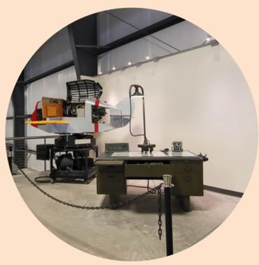
At the top of the stairs on the mezzanine, you will find a **Link Instrument Trainer**. A series of bellows, pumps, and valves allowed the trainer to simulate aircraft movement. Using the trainer was safer and cheaper, because the student wasn't using an actual aircraft that required fuel and maintenance. The Army Air Corps began using them in 1934 and implemented a hood, so the pilot would have to use the instruments in the "cockpit" to fly, and not rely on visuals while flying.
