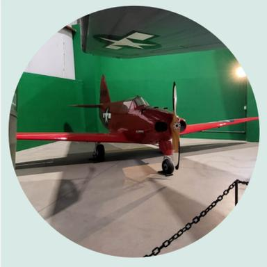
Behind the Skytrain is a small red plane, the **PQ-14 drone**. These all-wooden drones could be flown remotely or by a pilot. The remote feature meant that these were useful for target practice for anti-aircraft gunners in the US Navy and Army.
