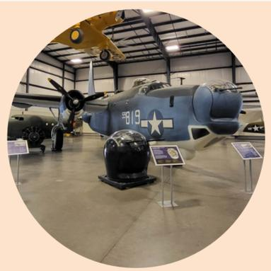
**The PB4Y-2 Privateer** is a long-range patrol bomber based on the B-24 Liberator. Some differences include a single tail, more armament, a stretched fuselage, and state of the art radar and navigation equipment giving them all-weather capability. They flew anti-submarine and anti-shipping missions in the Atlantic and the Pacific. After WWII, they also served as weather reconnaissance and signal intelligence gathering. Some served as aerial tankers fighting forest fires through 2002.
